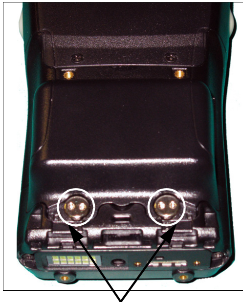
Secure Battery Cover Latches (in locked position)
