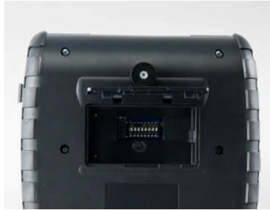
FIGURE 10: DIP SWITCH LOCATION
