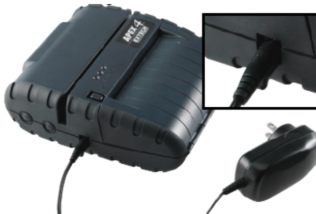
FIGURE 3: CHARGING THE BATTERY CARTRIDGE
