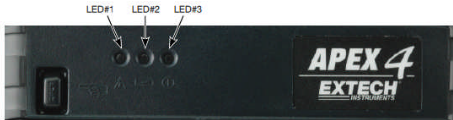
FIGURE 4 - LED INDICATOR LOCATIONS
