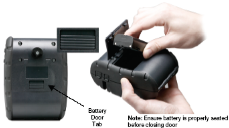
FIGURE 2: INSTALLING THE BATTERY CARTRIDGE
